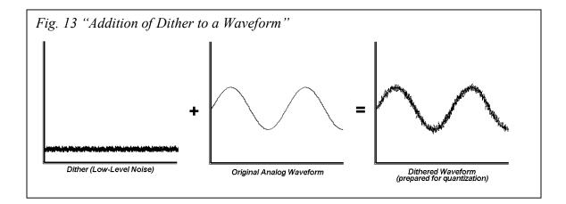
quantization error. In addition, since the dither is added by the ADC, it can be filtered in specific ways to ensure that it rests at intervals within the frequency spectrum where it is aurally masked. This technique, called noise-shaping, "re-equalizes the spectrum of the dither while retaining the power, effectively moving the noise away from the areas where the ear is most sensitive (circa 3 kHz), and into the high frequency region," as seen in Fig. 14 (Katz 55).
