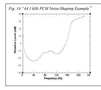
associated with sigma-delta modulation is very large, resulting in significant quantization noise;" however, unlike the PCM structures this "noise can be shaped such that virtually all noise power falls outside the range 0-20 kHz," well above the range of human aural perception
