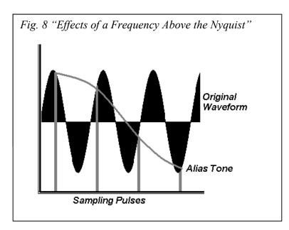
these common affects found in low-Q filters required for PCM, it is a logical step to reference the steepness of the anti-aliasing filter's slop when addressing the quality of a digital system. Of course, this slope is able to have a much lower Q when an ADC is able to utilize a larger frequency response, allowing the least amount of artifacts to be introduced to the audible incoming signal in audible regions.
