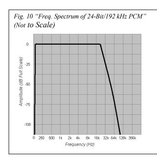
Unlike PCM filtering methods that utilize the entire bandwidth capable under the Nyquist theorem, DSD does not use all frequencies available within its system. Instead of encoding all frequencies below the Nyquist frequency of 1.4 MHz, a DSD
