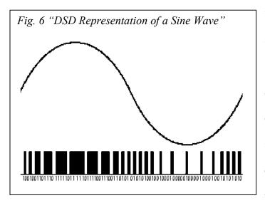
following the SDM, downsampling the one-bit output of the SDM to a multi-bit data stream to a form compatible with the needs of that specific PCM system or storage device (Fig. 3). In contrast, the DSD structure utilizes the SDM's one-bit output
